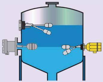
As shown above, if nstallation direction of the sensor is horizontal, the wiring penetrations must be facing down (Bottom). In addition, if the length of the flange pipes is long, during installation, the vertical movement of the float may not work properly so that check the specification of the tank and product.
