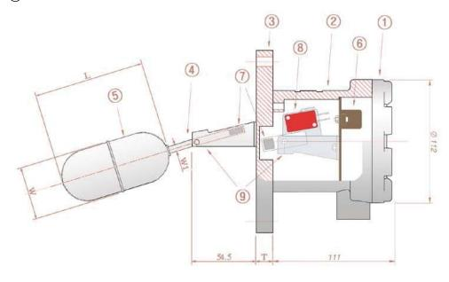
The level switch uses the force of repulsion between magnets of the same polarity. The float moves in the vertical motion according to the liquid level change.
