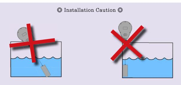
As shown in the picture, when you install DGS Sensor, if the wire is bent or warped, it could be the cause of the malfunction of DGS sensor. Please note that when installing.
