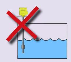
Install the sensor so that it is perpendicular. Float of the sensor does not touch the wall of the tank.
