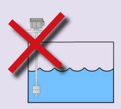
Install the sensor so that it is perpendicular.
