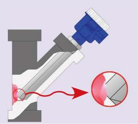
If any high viscosity liquid remains stick to the sensing part (Probe) as shown, it may result in malfunction of the product.
