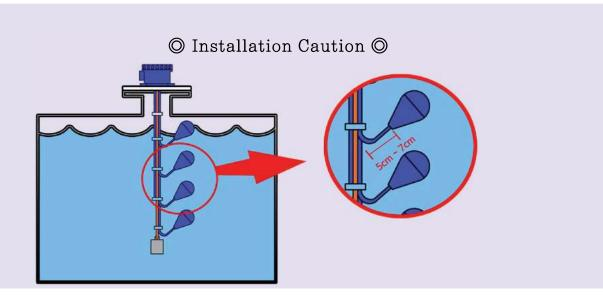
As shown in the picture, when you tie Quick float cable, be sure to connect with  $5 \text{cm} \sim 7 \text{cm}$  margin length at minimum. If there is no margin length, Quick float can not rise up so that it may cause a malfunction. The Weight should be installed not to touch the bottom of the tank.
