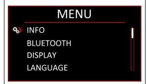
Push the "Down displacement" button until the prompt points to the Bluetooth option and then push the "Enter" button.
