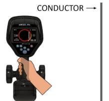
4. The signal starts decreasing so the direction of the rotation must be changed in purpose of returning to the maximum signal point.
