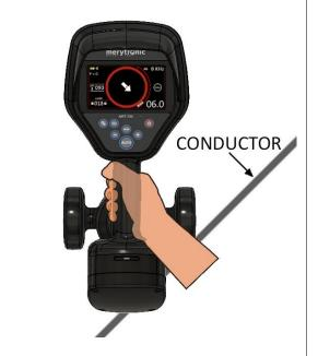
3. The signal is increasing and the 4. The conductor isn't in vertical position so conductor has appeared in the display so we'll have to rotate the tracer until we get we are doing right.
