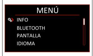
Push the "Down displacement" button until the prompt points to the Display option and then push the "Enter" button.
