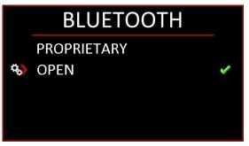
Once the protocol has been selected, in the menu, the option set BT pair will appear. We must select it to establish with the connection with the desired device.
