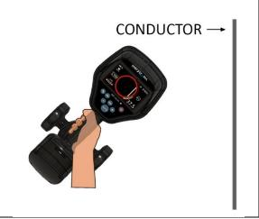
Once the MRT-700 is parallel to the conductor, we have to move to place just about it. For doing this, you must take notice of the positioning information that appears in the screen (viewfinder, signal quantity...) and then follow the next steps.
