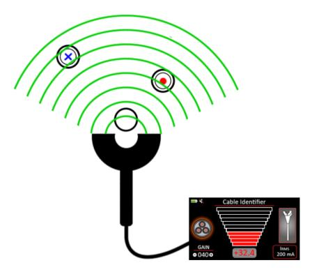
In spite of the fact that for the conductor in which the sensor is being placed in U, no current is circulating, the receiver is detecting a signal which can lead to an erroneous identification.
