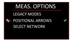
Activating this option means that arrows will appear in the viewer, in order to help to center the cable while tracing, regardless of the screen mode and frequency, as shown in the following image.
