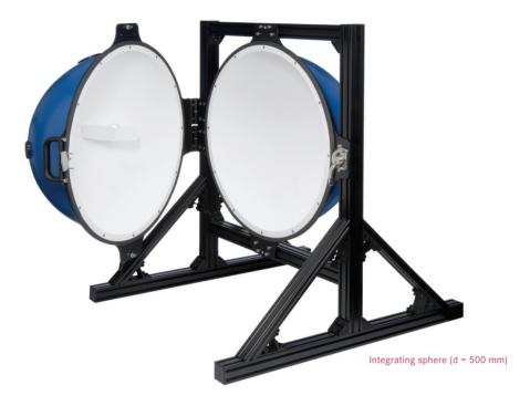
Integrating spheres distribute incident light by diffusing reflection evenly over the inner surface of the sphere. They are used in a variety of measuring applications for the integration of light and radiation and as a source of uniform diffuse radiation.
