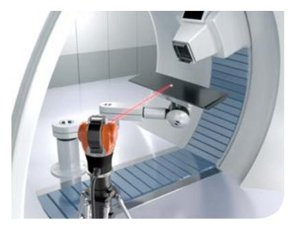
For corpuscular ray therapy apparatus, since millimeter accuracy is required for irradiating therapy zones, high accuracy is needed when setting the bed position and direction.
