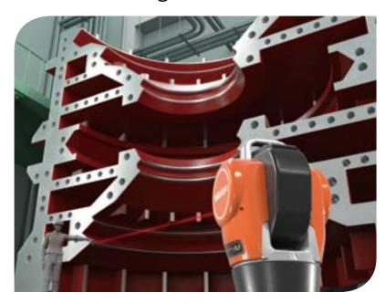
Accuracy to 0.1 mm is required for the inner diameter measurements of vapor turbine casings to obtain optimum efficiency of power generated by pressurization.
