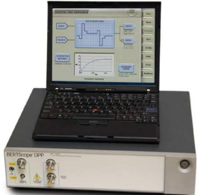
The BERTScope DPP Series can operate as a stand-alone instrument controlled by a PC, or with a BERTScope for complete software integration. It can be fully automated, and with its compact size, the DPP will easily fit into a manufacturing environment.
