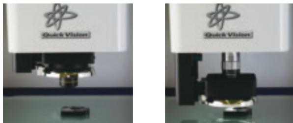
Measuring the top and bottom widths of metallization patterns on an IC package
