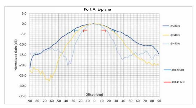
Figure 15: Typical antenna patterns at three different frequencies with Port A, E-plane
