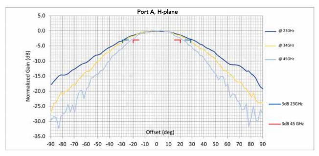
Figure 13: Typical antenna patterns at three different frequencies with Port A, H-plane
