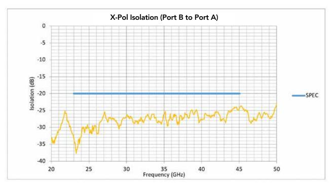
Figure 12: Cross Polarization Isolation Port B to Port A
