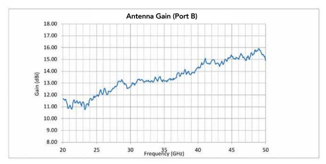
Figure 7: Antenna Gain, Port B
