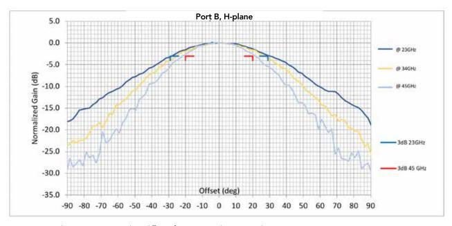
Figure 14: Typical antenna patterns at three different frequencies with Port B, H-plane
