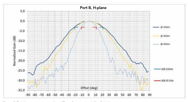
Figure 18: Typical antenna patterns at three different frequencies with Port B, H-plane
