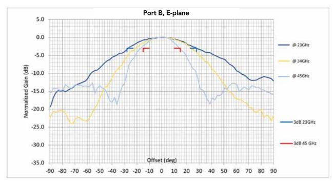
Figure 16: Typical antenna patterns at three different frequencies with Port B, E-plane
