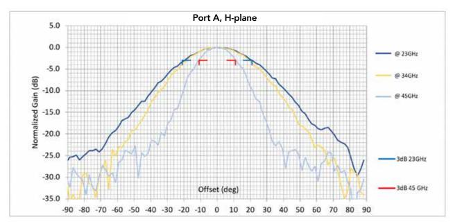
Figure 17: Typical antenna patterns at three different frequencies with Port A, H-plane
