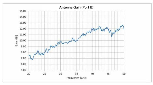
Figure 1: Antenna Gain, Port B
