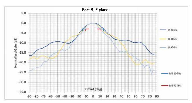
Figure 20: Typical antenna patterns at three different frequencies with Port B, E-plane
