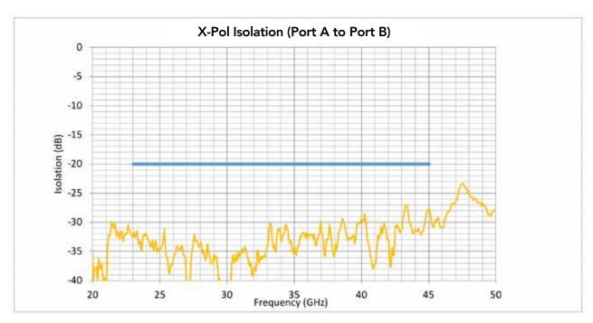
Figure 11: Cross Polarization Isolation Port A to Port B
