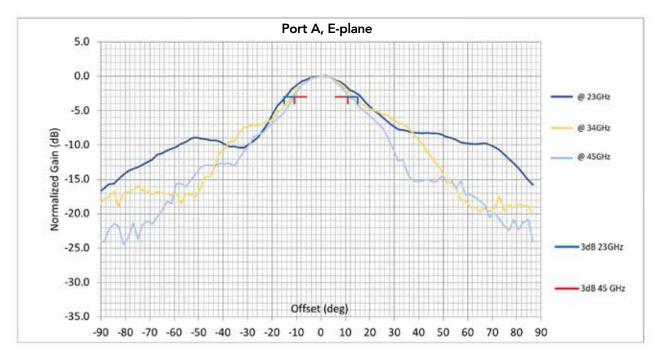
Figure 19: Typical antenna patterns at three different frequencies with Port A, E-plane
