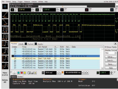
Trigger and view on-screen serial decode of I 2 C packets.
