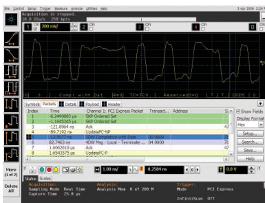
Trigger on and decode PCIe serial packets.
