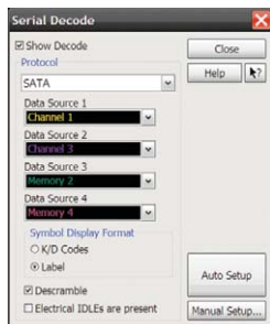
Trigger on and decode SATA serial packets
