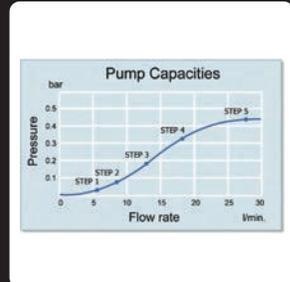
Five speed duplex pump is easy to control pump capacities and pressures (only for CW, RW models)
