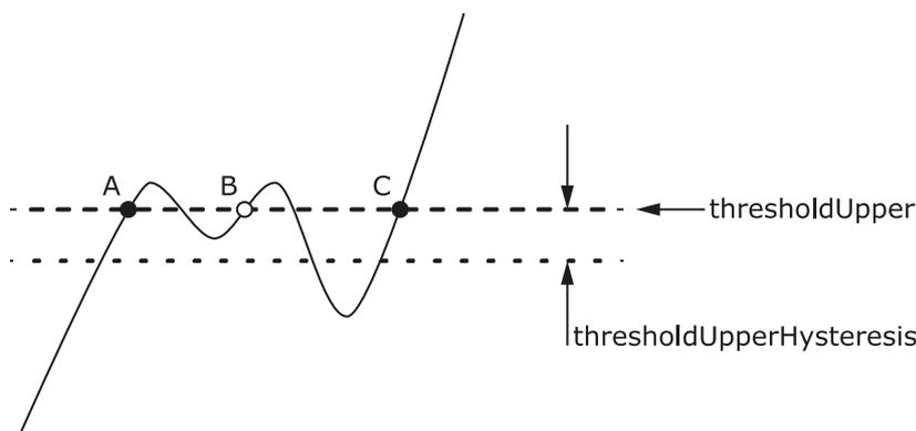
**Hysteresis** – The trigger fires at **A** as the signal rises past both thresholds. It does not fire at **B** because the signal has not passed the hysteresis threshold. The trigger fires again at **C** after the signal has dipped below the hysteresis threshold and risen past both thresholds.
