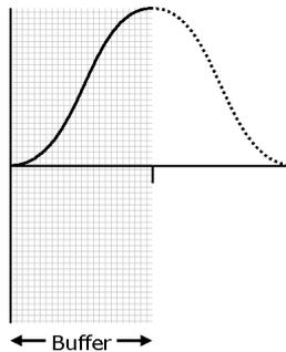
**QUAD mode.** The generator outputs the contents of the buffer, then on its second pass through the buffer outputs the same data in reverse order as in dual mode. On the third and fourth passes it does the same but with a negative version of the data. This allows you to specify only the first quarter of a waveform with fourfold symmetry, such as a sine wave, and let the generator fill in the other three quarters.
