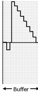
**DUAL mode.** The generator outputs the contents of the buffer from beginning to end, and then does a second pass in the reverse direction through the buffer. This allows you to specify only the first half of a waveform with twofold symmetry, such as a Gaussian function, and let the generator fill in the other half.
