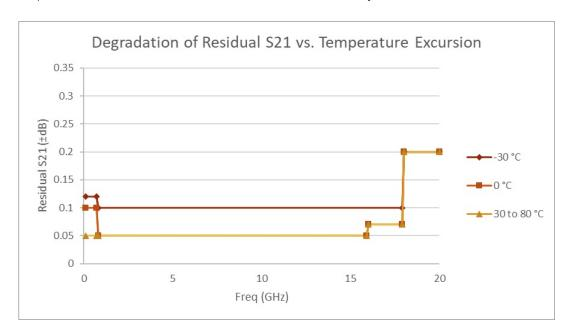
Table 8 Residual Recorrection Errors Versus Temperature Change
