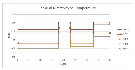
Table 22 Residual Recorrection Directivity Errors Versus Temperature Change
