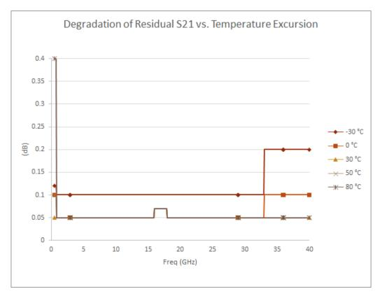
Table 21 Residual Recorrection Errors Versus Temperature Change
