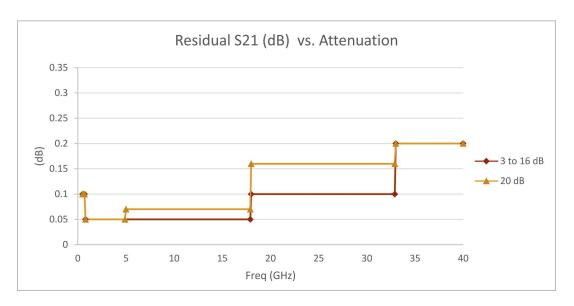
Table 15 Residual Recorrection Errors of S21 and S12 Magnitude Versus Attenuation - 85540B/1B/2B
