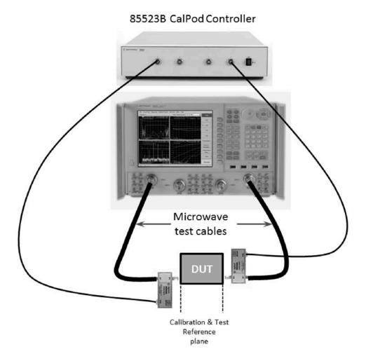
The measurement uncertainty of a CalPod recorrection of a 2-port DUT can be determined by adding the recorrection residual S21 error of CalPod 1 and the recorrection residual S21 error of CalPod 2 together. The tables and graphs in this document provide values for the recorrection of residual S21 error versus frequency for the different models of CalPods.
