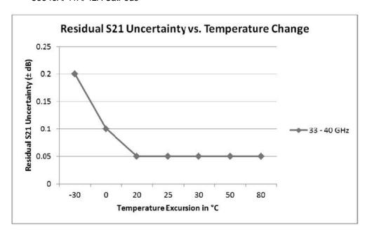
Figure 3 Example: Temperature Change Effects and Temperature Hysteresis Effects for 85540A/41A/42A CalPods
