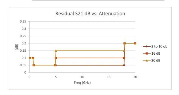
Table 5 Residual Recorrection Errors of S21 and S12 Magnitude Versus Attenuation - 85530B/1B/2B
