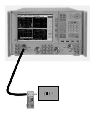
When using a CalPod in a measurement system for a 1-port DUT, the residual directivity of the CalPod limits and defines the lowest reflection that can be resolved with the measurement system. Mathematically, the residual directivity can be defined as:
