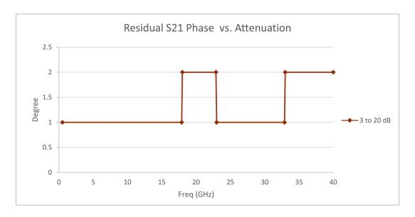
Table 16 Residual Recorrection Errors of S21 and S12 Phase Versus Attenuation - 85540A/1A/2A
