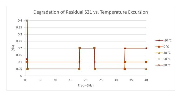
Table 20 Residual Recorrection Errors Versus Temperature Change
