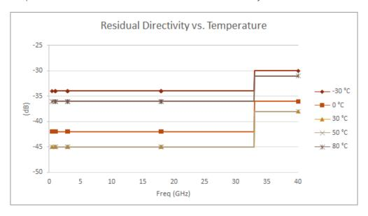
Table 23 Residual Recorrection Directivity Errors Versus Temperature Change
