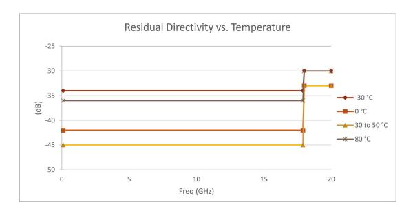
Table 9 Residual Recorrection Directivity Errors Versus Temperature Change
