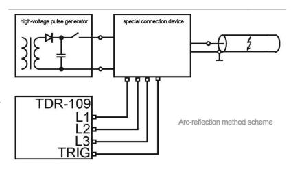
low resistance of the arc with inverted polarity (like shorted circuit waveform). The method does not require the prior isolation burning and particularly effective when working on polyethylene sheath.
