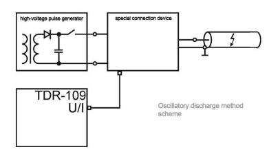
which has a small resistance, and the oscillatory discharge proceeds. Knowing the speed of propagation of electromagnetic waves along the cable and the period of oscillations process, we can calculate the distance to the breakdown:
