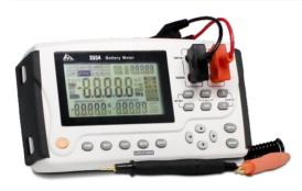
The 3554 battery tester is designed for large current and strong anti-interference to provide fast, complete and accurate diagnosis in internal resistance and voltage for backup UPS batteries and lead-acid batteries. Without stopping the instrument, 3554 can carry out online measurement and rapid diagnosis of deterioration of the batteries, greatly increasing the test efficiency. The built-in automatic data storage function can store up to 2400 sets of data.
