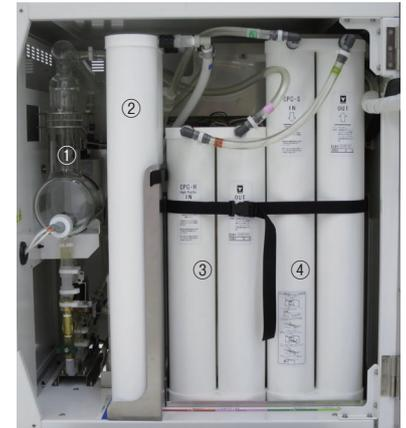
Most consumable parts, including the Ion exchange resin cartridge, High purity cartridge, Pretreatment cartridge can be easily attached and detached, facilitating easy maintenance work.
