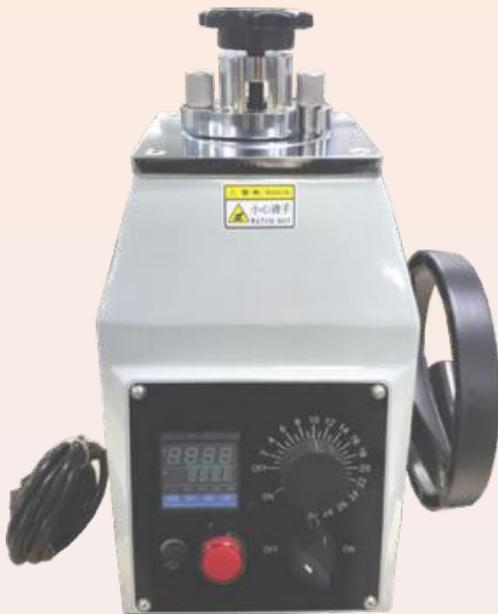
MP-1 metallographic sample mounting press is designed for mounting small or irregular shape and those difficult to hold samples, which is former procedure of grinding and polishing. The inlaying operation serves to facilitate the grinding and polishing operations of the specimens and the routine observation of the composition of the material under the metallographic microscope.
