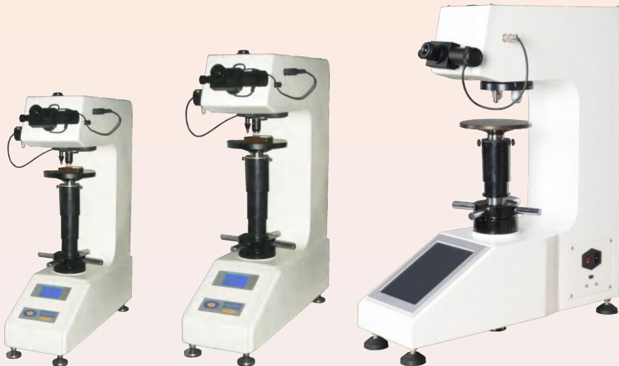
Digital eyepiece with inbuilt encoder, automatic calculate, high accuracy & easy operate.
