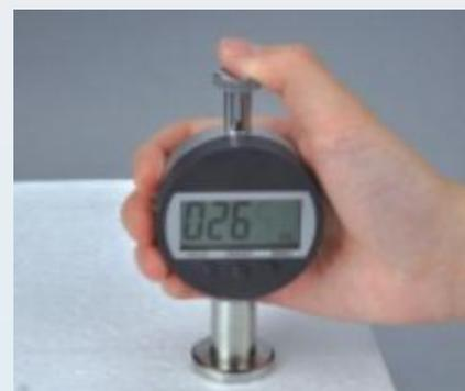
**IRHD Hardness Testers - International Rubber Hardness Degrees**
