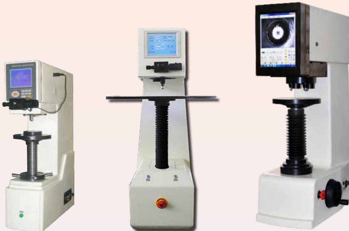
Press one key machine will automatic rise work table - loading - dwell - unloading
