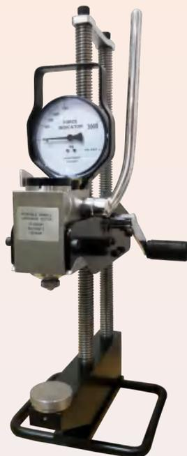
Standard parts come with 20X reading Microscope; With LED light, indentation image more clear and easier to measure
