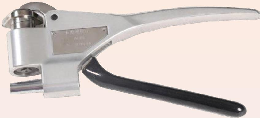
Webster hardness testers also known as Webster hardness pliers; they can be used to test the hardness value of aluminum alloy quickly at the scene of the production. They are the preferred instruments for testing the force of aluminum alloy.
