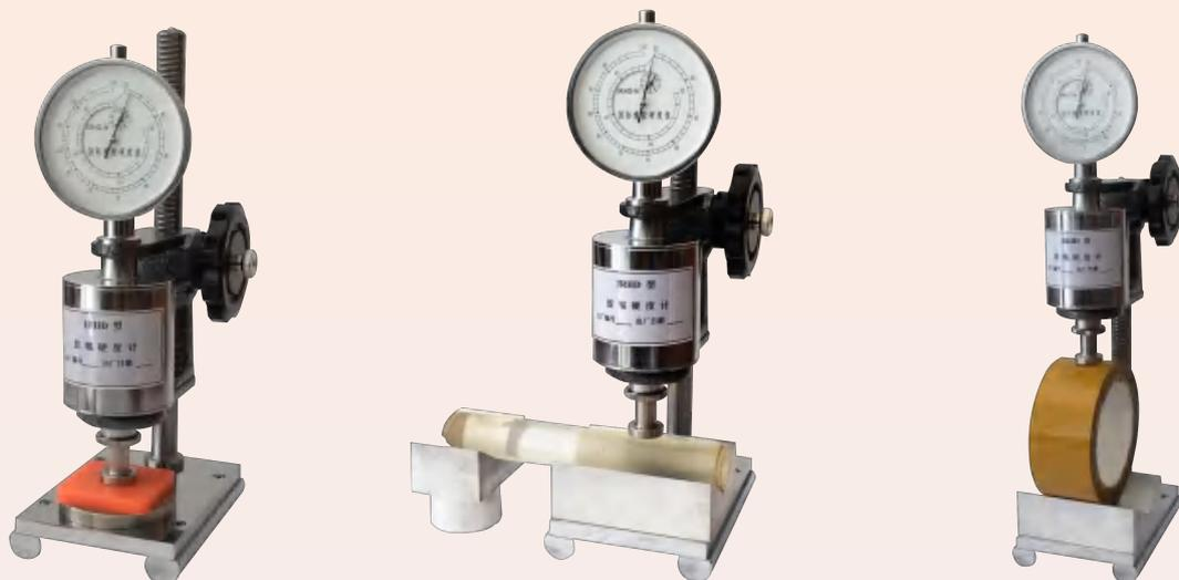
This instrument is used to measure the hardness of rubber and similar rubber materials, especially suitable for measuring the hardness of rubber rollers, hoses, cables and rubber products with curved structures. This hardness tester has simple structure, convenient operation, accurate measurement, intuitive reading, and can directly calibrate the international standard rubber hardness value (IRHD) of the sample.
