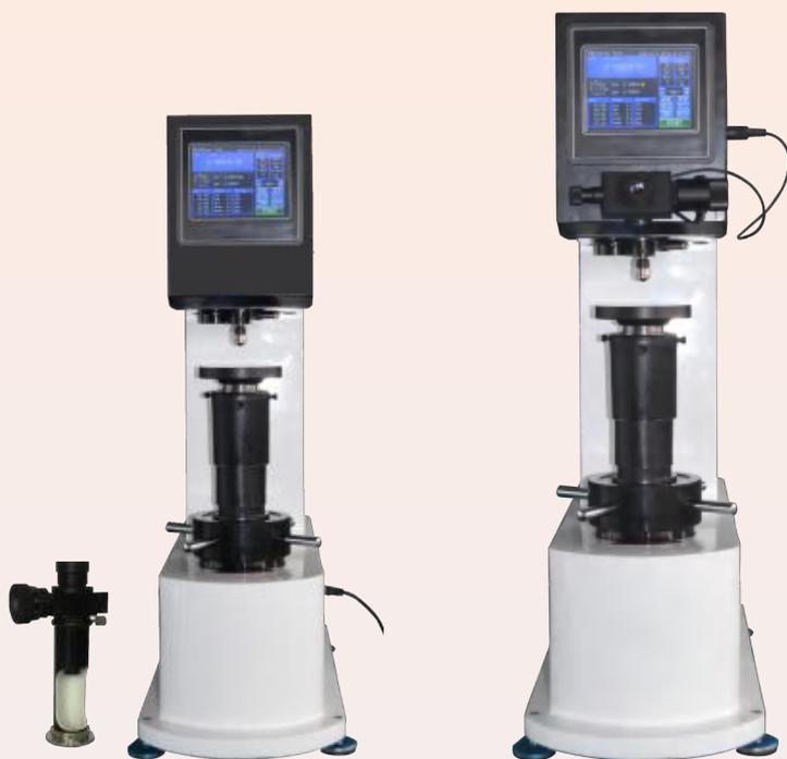
**eBRI-3000:** input the indentation diameter length to screen, machine will auto calculate and display Brinell value on screen
