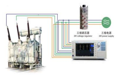
The accuracy measurement of power transformer
