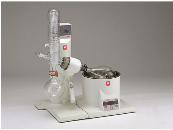
The photo shows RE 301 B-O (main body + glass set B + oil bath BO 400 type)
