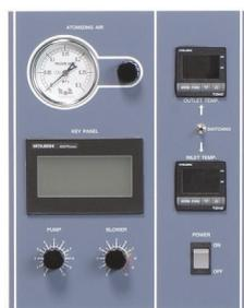
Inlet temperature, outlet temperature, and drying air amount are digitally displayed. Setting is made on the touch panel that allows operation settings, operation status displays as well as error display, and settings of various operation conditions. as well as error display, and settings of various operation conditions.
