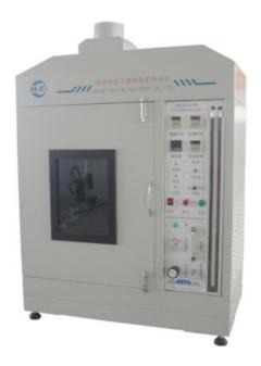
Designed according to the UL94 standard, the ignition risk of household appliances, parts and components of electrical and electronic products is assessed mainly by analog technology measurement.
