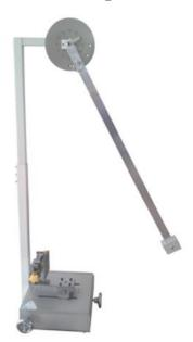
Designed according to APPLE's special requirements, it is mainly used to test the impact resistance of the APPLE adapter. The length, size and weight of the pendulum are designed in strict accordance with APPLE requirements, and the angle can be selected according to the test requirements.
