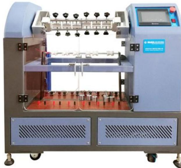
The load bending testing machine is a special equipment for testing the bending fatigue strength of various power lines, connectors, wires, terminals, laptop power adapters, etc. This machine can measure six samples at the same time. This machine adopts PLC+ servo system + touch screen control, with the characteristics of accurate positioning and high precision.
