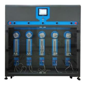
The bending tester is a special equipment for testing the bending fatigue strength of various power lines, connectors, wires, terminals, laptop power adapters, etc. This machine can measure six samples at the same time. This machine adopts PLC+ servo system + touch screen control, with the characteristics of accurate positioning and high precision.
