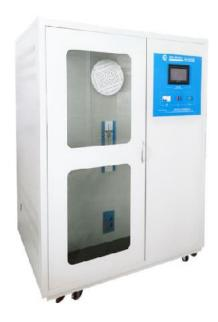
Mainly used for testing the bending fatigue strength of ac power cord and plug lead. Suitable for testing the swing motion of the power cord of plug under certain load.
