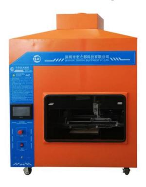
This instrument is mainly used to test the flame resistance test of non-metallic materials and finished products, and is applicable to the industry or place of the fire resistance test project of the quality inspection department and related manufacturers.
