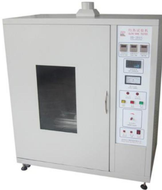
The test equipment consists of a box body, an exhaust vent, a glow wire, a flame height gauge, a current control system, a temperature control system, a horizontal moving trolley, a sample fixture, a fixed/timer device, a residue tray, a white pine board, and a paper. Weight and other components.
