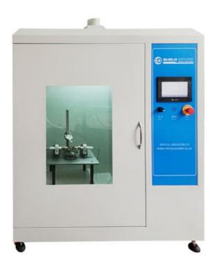
This instrument is mainly used to test various solid insulating materials used in electric and electronic equipment. Under the combined action of electric field and contaminated medium, the surface may gradually form conductive passages due to tracking, which may cause electrical short circuit accident and cause fire. An important indicator that jeopardizes the reliable operation of equipment and personal safety.
