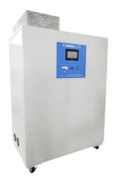
According to the technical requirements of U L1054 and relevant international standards, it is mainly used for the load live test of passive products between power supply plug wires, plugs, switches and contact wires. The testing machine has the advantages of beautiful appearance, reasonable layout, stable and reliable performance and convenient parameter setting.(large current) testing machine.
