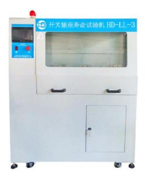
It is applicable to the breaking capacity and life test of plug and socket and the on-off ability and life test of switch. It can be combined with the company's load unit to form a closed-loop load power-on test system to make plug and socket or switch conduct simulated aging power-on test under critical environment.
