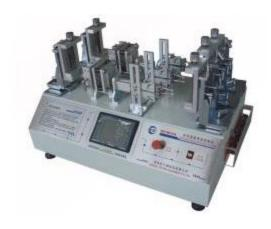
It is applicable to the breaking capacity and life test of plug and socket and the on-off ability and life test of switch. It can be combined with the company's load unit to form a closed-loop load power-on test system to make plug and socket or switch conduct simulated aging power-on test under critical environment.
