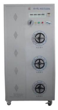
It is mainly used to test the overload test and durability test of passive products between power plug wires, plugs, various switches and various contact conductors.
