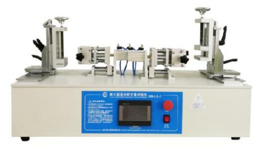
This test machine is suitable for the breaking capacity and plug life test of plugs and sockets. It can be combined with the load machine of our company to form a closed-loop load energization test system, so that the plug and socket can simulate the aging energization test under critical environment.
