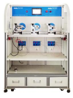
It is suitable for testing the service life of the plug wire under the condition of being perpendicular to the plane or rotating at a 45 degree taper, and simulating the service life of the tested product under certain load and load conditions. The external load port can be connected to the external load test product. Load test.
