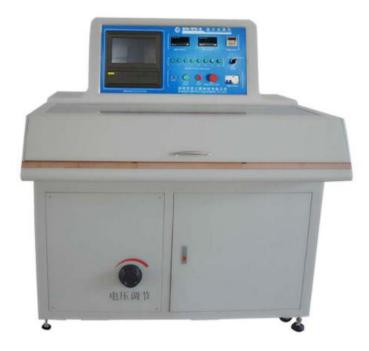
It is suitable for the current-resistant load temperature rise test of plug power cord. It adopts imported color temperature paperless recorder and computer to control display, record temperature change, output report and print, adopt integrated design.
