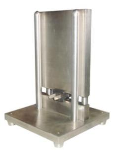
It is used to measure the pressure resistance of electrical accessories at high temperatures (80 °C  $\pm$  2 °C). The device consists of two steel clamps, each with a cylindrical surface with a radius of R25mm. During the test, a load of 20 N was applied to the object to be measured by the above clamp. The device has the advantages of simple structure, reasonable design and beautiful appearance.
