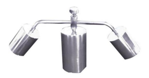
The ball pressure device is an insulating material device designed to maintain the current-carrying parts and the components of the grounding circuit in a normal position according to various technical requirements of the national standard. The device has a spherical diameter of 5 mm and applies a load of 20 N to the object under test during the test. The utility model has the advantages of simple structure, reasonable design, beautiful appearance and good reliability.
