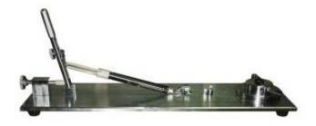
This instrument is mainly used to test the degree of tension of the coupler, and is suitable for testing whether the coupler with rated value greater than 0.2A is damaged under the corresponding tension. The tension part adopts the pointer type spring balance, which is accurate in measurement, convenient in observation and record, practical and reliable.
