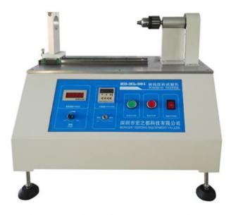
This machine is mainly used for copper wire torsion test. When testing a certain torsion speed, how many times the copper wire is twisted.
