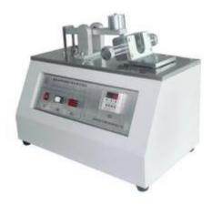
This instrument is mainly used to test the wear resistance of the plug and sheath insulation sheath. The utility model has the advantages of compact structure, beautiful appearance, reasonable layout, convenient use and maintenance, and the like.
