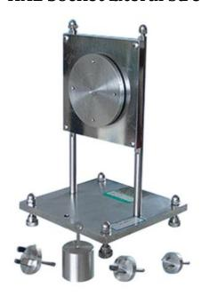
The device is suitable for the lateral stress applied to the electrical appliance inserted into the socket for a socket or converter with a rated current of not more than 16A and a voltage of not more than 250V.
