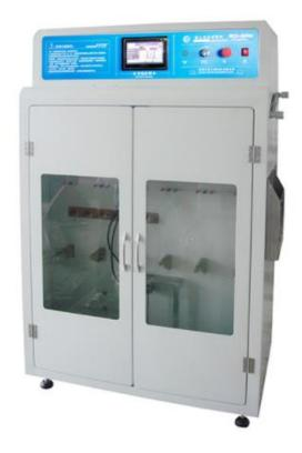
The instrument is suitable for the tensile strength test, torsion test, load test and grounding wire current test of the conductor wire between the plug piece and the conductor of the power plug wire. The instrument adopts touch screen and PLC control, and has the advantages of beautiful appearance, reasonable layout and convenient maintenance.
