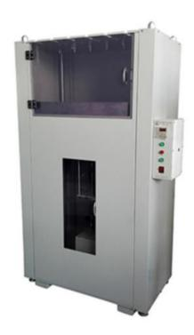
This instrument is suitable for testing the impact resistance of plugs and sockets.
