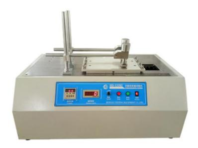
It is used to test the abrasion resistance of the printing ink layer and the abrasion resistance of the surface coating. It effectively analyzes the anti-friction properties of the printed matter, the drop of the ink layer, the hardness of the coating, etc., and automatically records the number of frictions.
