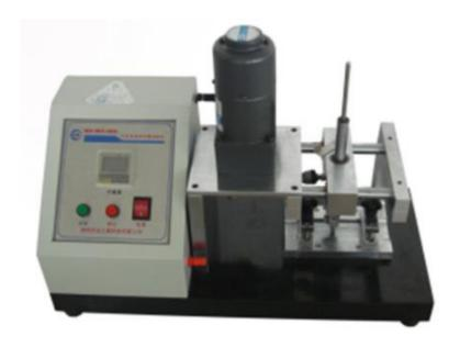
This instrument is mainly used to detect the scratch resistance of automotive low voltage wires.
