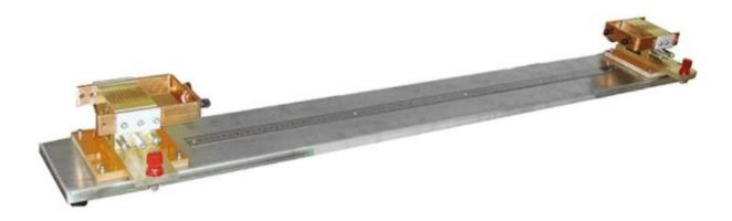
This fixture is mainly used to measure the DC resistance of the conductive core of wire and cable with the bridge tester. It can measure the DC resistance of round wire, stranded wire, flat wire and fan wire. It can also be attached to the terminal to measure various specifications of enameled wire below 0.1 mm.
