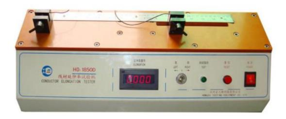
This product is only used for the elongation of annealed copper wire below 1.0mm, and is suitable for the elongation test of various linear metals by manufacturers and quality inspection departments.
